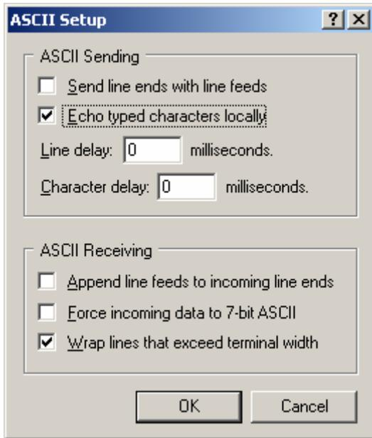
After all this you can enter AT commands in the large white area of Hyperterminal. You should see a cursor. When you press the ENTER key, the command will be sent to the modem. If you make a mistake, press ENTER and retype the command. Be sure to turn result codes and echo modem commands OFF ("Q1" command, quiet mode enabled and "E" command) before exiting HyperTerminal.
